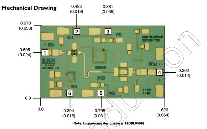
Units: millimeters (inches) Bond pad dimensions are shown to center of bond pad. Thickness: 0.115 +/- 0.010 (0.0045 +/- 0.0004), Backside is ground, Bond Pad/Backside Metallization: Gold All Bond Pads are 0.100 x 0.100 (0.004 x 0.004).
